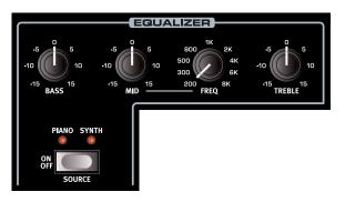
The three band equalizer features bass, sweepable midrange and treble controls.
