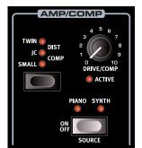
The **AMP/COMP** unit includes sophisticated amplifier and speaker cabinet simulations, a versatile tube distortion setting and a useful compressor effect. The amount of drive or compression is controlled with the **DRIVE/COMP** knob. The LED indicates whether any overdrive is active, and will light up whenever the compressor is working.
