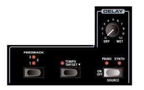
The **DELAY** unit produces echo/repeat effects. The Delay time is set by tapping the **TEMPO** button, or by pressing down on it and **SET** the tempo using the Program section dial.
