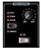
The **REVERB** unit simulates the natural sound reflections in various acoustic environments. The Reverb is a "global" effect, which is to say that it is always applied to *all* active sound engines.
