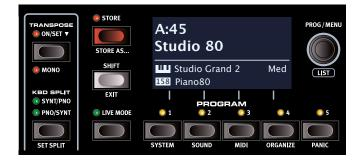
The centrally located Program section provides access to performance functions such as loading and storing programs, access to Live programs, keyboard split functionality and more. This is also where menus containing *System, Sound* and *MIDI* settings are found. The menus and their settings are covered in a separate chapter, starting on page 22.
